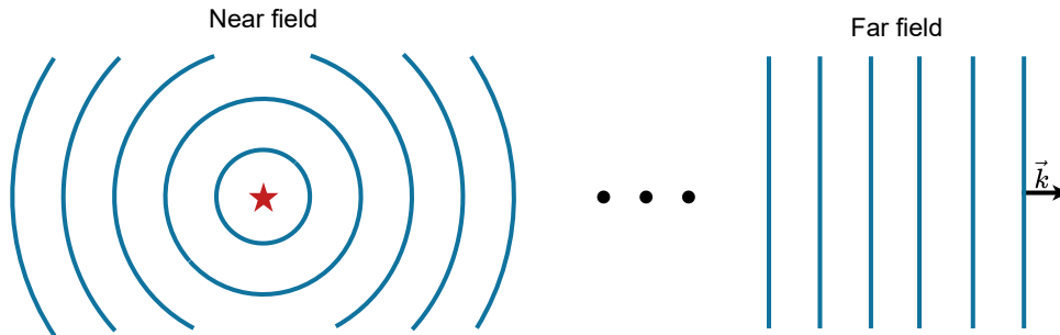
Fig. 2.2: Spherical waves are used to model waves in the near field, while plane waves are used to model waves in the far field. Vector \vec{k} is parallel to the direction of propagation at each point.
